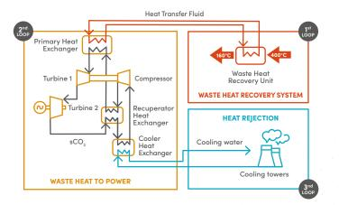
CO2OLHEAT's WH2P application is based on a recuperated closed-loop Brayton cycle with sCO<sub>2</sub> as a working fluid. Thanks to its flexibility (compact size and capability to better accommodate load changes), high efficiency, and the ability to work with significant temperatures, the sCO<sub>2</sub> power block offers benefits beyond traditional WH2P applications.
