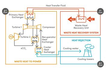
CO2OLHEAT's WH2P application is based on a recuperated closed-loop Brayton cycle with sCO as a working fluid. Thanks to its flexibility (compact size and capability to better accommodate load changes), high efficiency and the ability to work with significant temperatures, the sCO<sub>2</sub> power block offers benefits beyond traditional WH2P applications.
